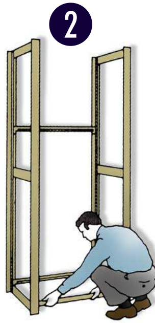
2 BUILD FROM THE BOTTOM UP Place shelf supports or quick-base (front and back) for lowest shelf only.
