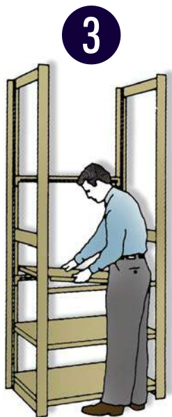
3 FIT SHELF OVER SUPPORTS Then add two more supports at the next shelf location, place shelf, and continue up the unit.
